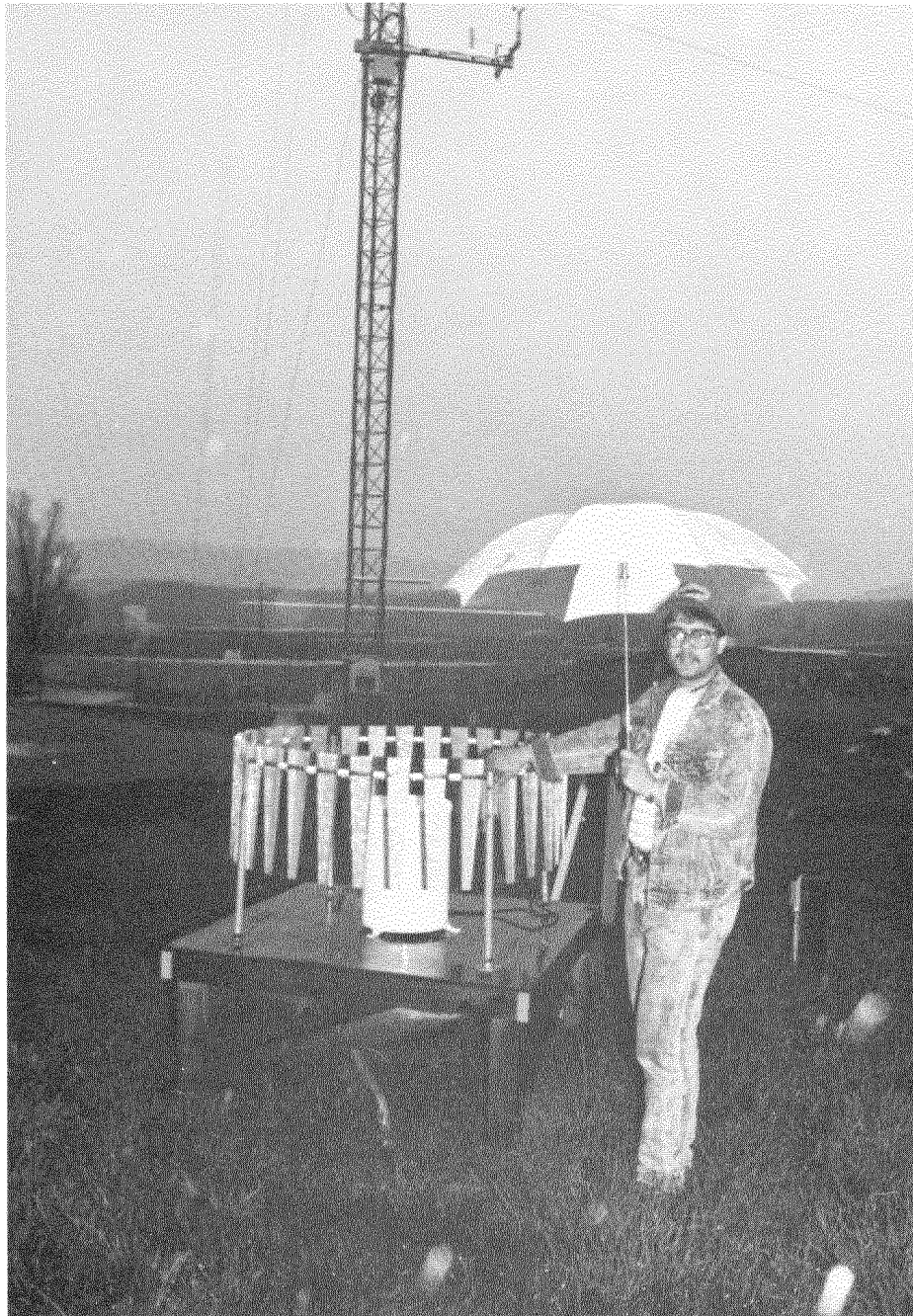
On-site Meteorological Tower and Rain Gage
