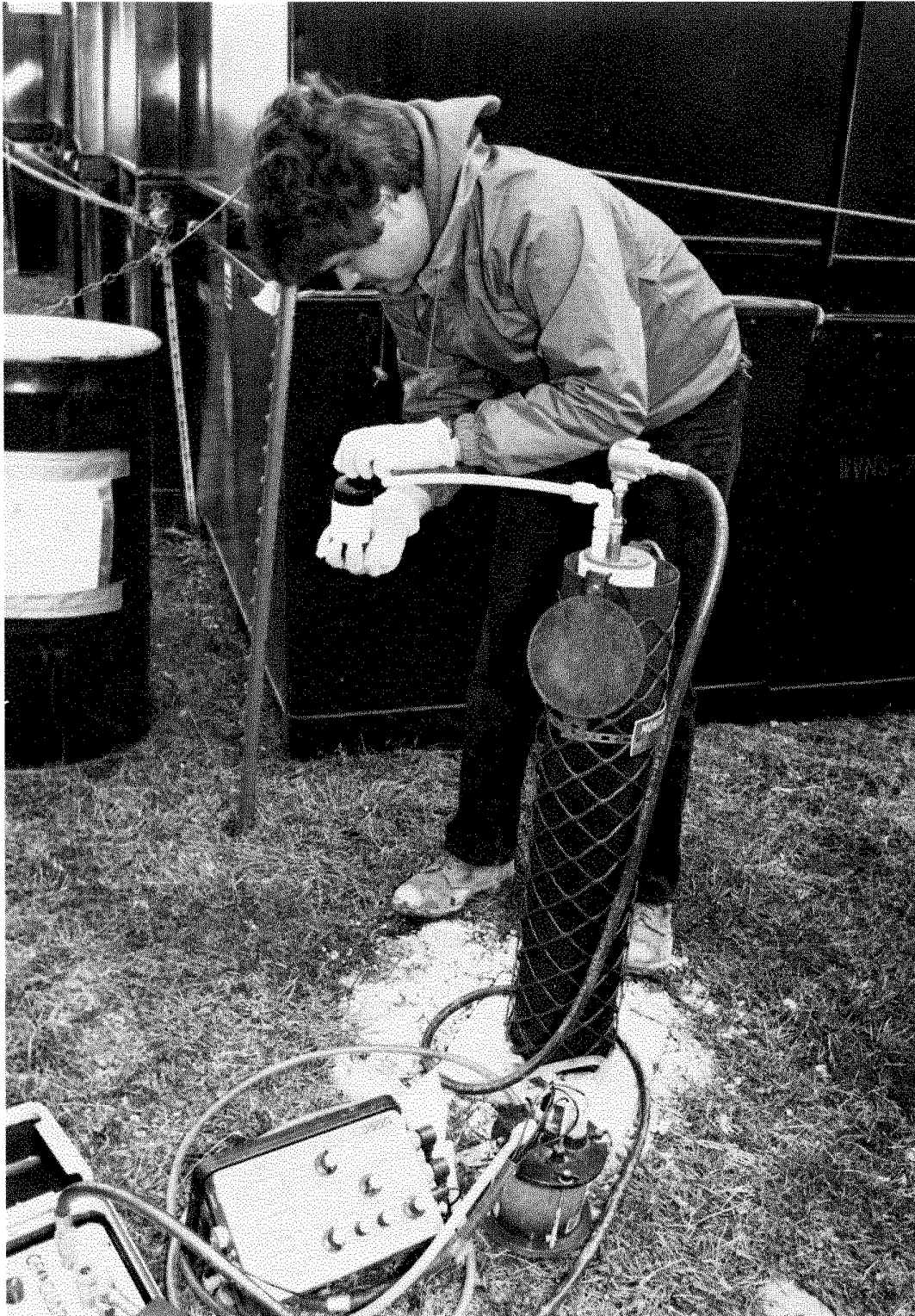
Sampling with a Dedicated Bladder Pump Installed in an On-site Groundwater Monitoring Well
