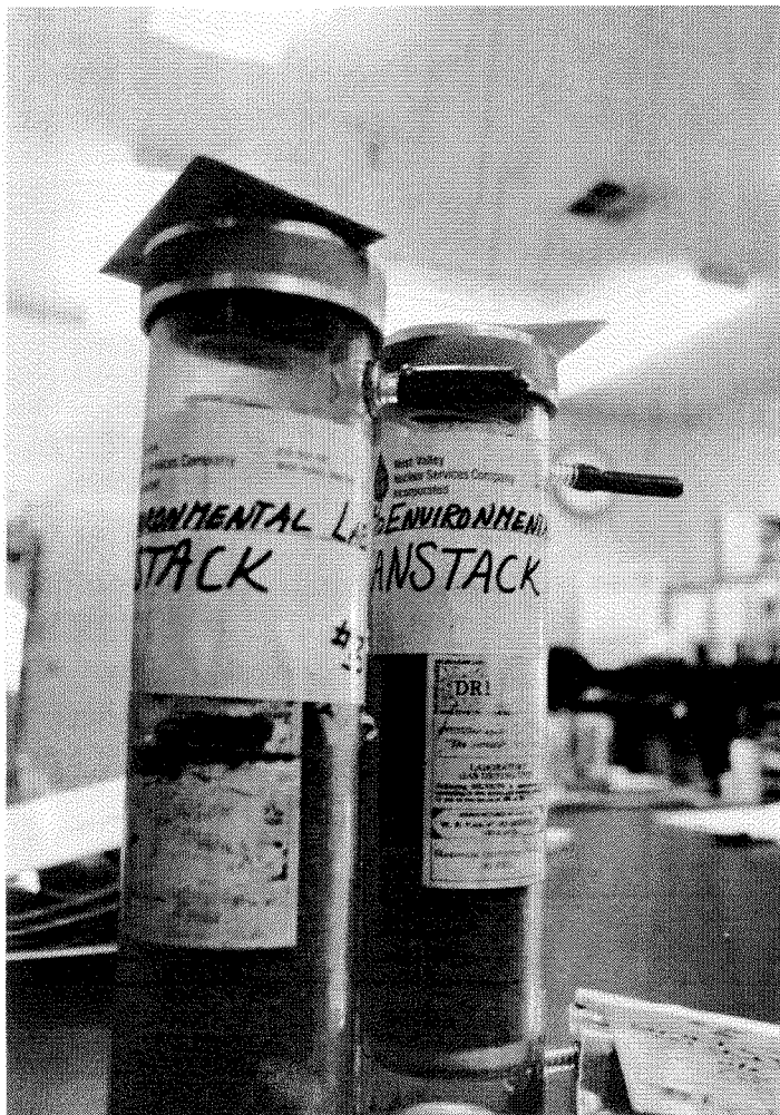
Silica Gel Columns from the Main Ventilation Stack Sampler
